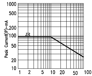
Fig6. MAX. PEAK CURRENT VS. DUTY CYCLE % (REFRESH RATE 1KHz)
